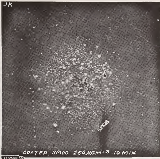
Figure 7. 100X SEM of impaction area of smog sample.
